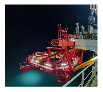
Our in-house product development has led to several patent pending innovations; for example the ability to safely catch the swinging monopile with the gripper, accurate positioning on the target location and dealing with a wide range of soil conditions during pile driving.
