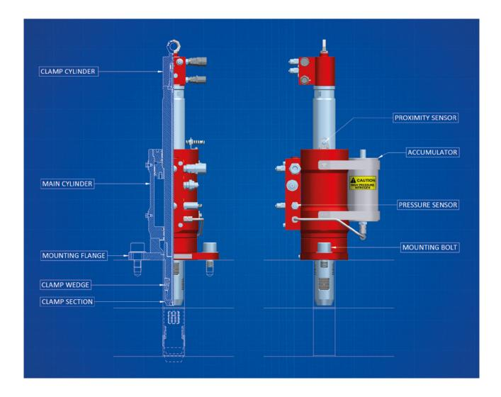
Flange Clamp Tools are used to temporarily secure the axial connection between the flanges of tower and substructure of a wind turbine generator prior and during the installation of permanent bolting. After installation of the majority (or all) of the installation bolts, all FCTs are removed.
